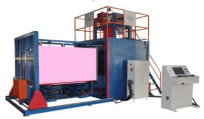
SL-VF-S Automatic vacuum foaming machine, adopt batching technology, foaming in vacuum condition. It is composed of storage tanks, batching, mixing, vacuum, mould, and computerized controlling systems. It can be realized numerical control during the whole production. It is used for making all kinds of foam.
